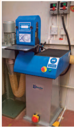
this machine shows that the sanding area can be minimized through adjusting the guard
