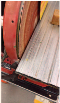
ensure gap is as small as possible between the table and the rotating disc, this machine also shows loose sanding material and no facility to minimize the sanding area
