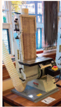
this machine has limited guarding, meaning too much of the moving sanding material can be accessed by users, thereby increasing the risk of catching fingers on the moving belt
