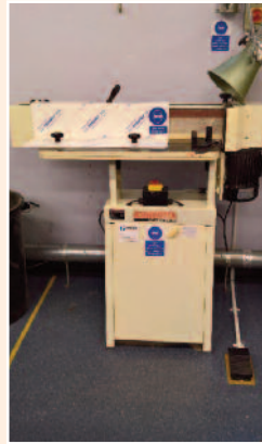
the school has designed and made a guard for this machine to limit access to the moving belt
