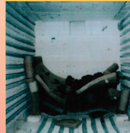
'Meltdown' resulting from an overnight firing without a secondary independent over-temperature protection systems (Heatfuse) Collapsed & bunched heating elements well past their "change by" date and probably working at less than 25% efficiency
