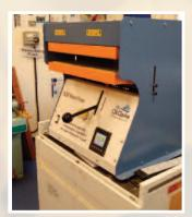
The process of chipping does not present any particular hazards, as long as the machine is used as specified by the manufacturer. However, the heating under pressure does create significant fumes, so must be carried out with extraction, or with good ventilation. The heated trays and equipment also present burn hazards, as does the heated plastic.
