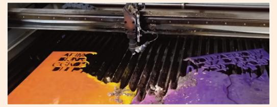
Our guidance is clear on the use of laser cutters; they must never be left unattended in use. We are making small changes to the relevant MRAT to make this, and other related points, completely clear:
