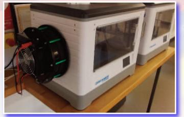
The benefit of using a cabinet, is that there are no drafts because the air around the build area is not disturbed. However, a cabinet is a large piece of equipment, whereas a small extractor may be less obtrusive. As the school decided to work with small extractors staff had to work through some constraints:
