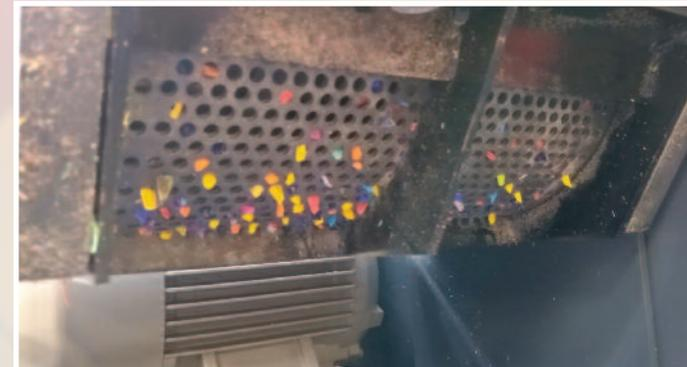
filled, there is no chance that the operator can get caught in the rotating blades. When the machine is being cleaned the operator can rotate the blades by hand, which does present a significant risk, so cleaning must only be carried out by trained and competent persons.
